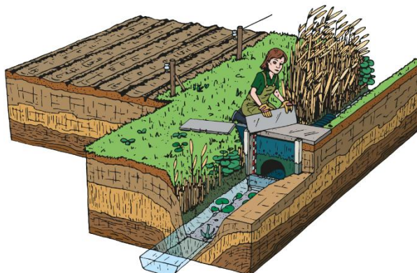
Figure 2: When you want the weir to have a draining function (i.e. during field work to prevent soil damage), you open the weir.
