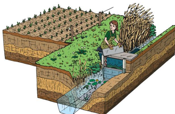
Figure 1: The adjustable weir is closed when you want the ditch to have an infiltration function.
